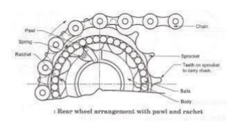
Power Train of a bicycle: The power train of a simple bicycle consists of a pair of pedals, two sprockets and a chain. The pedals are affixed to one sprocket — the front sprocket, which is
