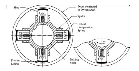
• A centrifugal clutch is a clutch that uses centrifugal force to connect two concentric shafts, with the driving shaft nested inside the driven shaft.
