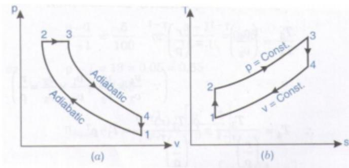
Processes : 1-2 : Isentropic compression 2-3 : Heat addition at constant pressure 3-3 Isentropic expansion 4-1 Heat rejection at constant volume
