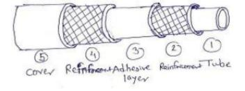
Pneumatic hose is made of several layers with metal wire braiding between them.
