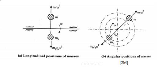
Fig. shows single rotating mass 'm' which is attached to a shaft rotating with angular velocity 'ω'.
