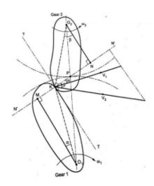
Consider the portions of two gear teeth in mesh. O1 and O2 are centre points.
