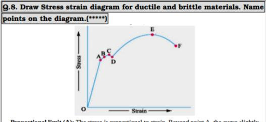
**Proportional limit (A):** The stress is proportional to strain. Beyond point A, the curve slightly deviates from the straight line. It is thus obvious, that Hooke's law holds good up to point A and it is known as Proportional limit.
