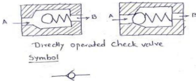
oil to flow. Hence oil can flow from port A to port B. when under pressure is supplied in opposite direction that is to port B, the oil force the ball to sit firmly in its seat, hence the passage is closed by ball. The oil cannot flow port B to port A.
