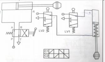
Working: In the first position of lever of 4/2 DCV (5/2 DCV can be used), the DAC extends. By the end of extension of first DAC, the cam presses roller of valve LV1 hence compressed air flows to second DAC, and second DAC extends. When the lever of 4/2 DCV is shifted to second position, DAC retracts. By the end of retraction of first DAC, the cam presses roller valve LV2, hence compresses air flows to second DAC and second DAC retracts.
