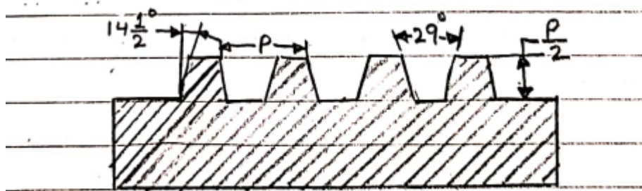
Fig: Acme Threads.
